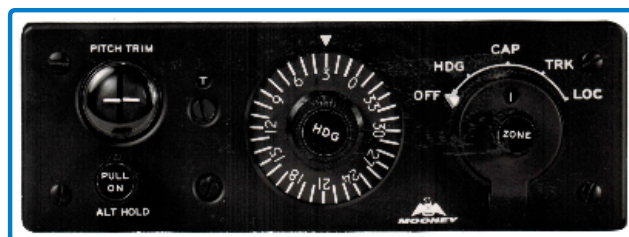
Brittain Model BI-601 Controller - this controller was used with both the B6 system and the Nav 2B system with the pitch indicator blanked out.
